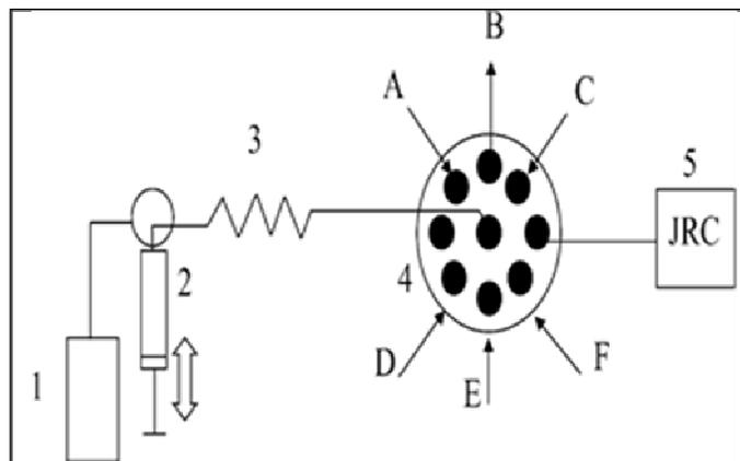
**Figure 1.** Schematic diagram of the SIIA system showing (1) carrier solution, (2) syringe pump, (3) holding coil, (4) multi-position valve (connecting (A) bead suspension, (B) waste out, (C) bleach solution, (D) sample solution, (E) labelling solution and (F) substrate solution and (5) jet ring cell.
